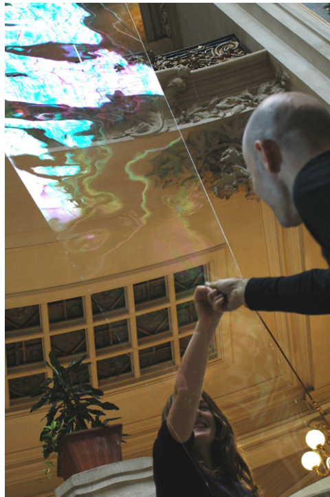
Figure 5. The curtain is robust enough to pass across it a finger, a hand or an arm (wet with water and dishwashing liquid). This particular curtain was 18 m high and the handshake lasted for more than 30 s [4]. Photo O Gatine.
