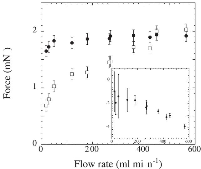
FIG. 2. Forces exerted by the flowing foam on the airfoil versus flow rate: drag ( $\square$ ) and lift ( $\bullet$ ). Inset: leading angle ( $\circ$ ) spontaneously selected by the airfoil versus flow rate ( $\text{ml min}^{-1}$ ); the standard deviation of its time fluctuations are plotted as error bars.
